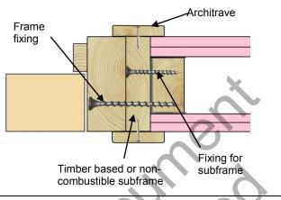
5. Timber based or noncombustible subframe up to 50mm thick, with gaps up to 10mm between components filled on both sides with 10mm depth of acrylic intumescent mastic or full depth expanding PU foam, fire tested for this application to BS 476: Part 22: 1987 or BS EN 1634-1. Joint must be fitted with 15mm thick overlapping architraves least 15mm each side.
